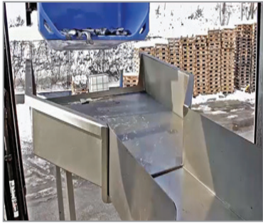
Fig. 3.1.7. Feed chute and receiving table
