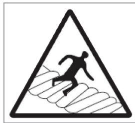
Danger Fragile Roof
